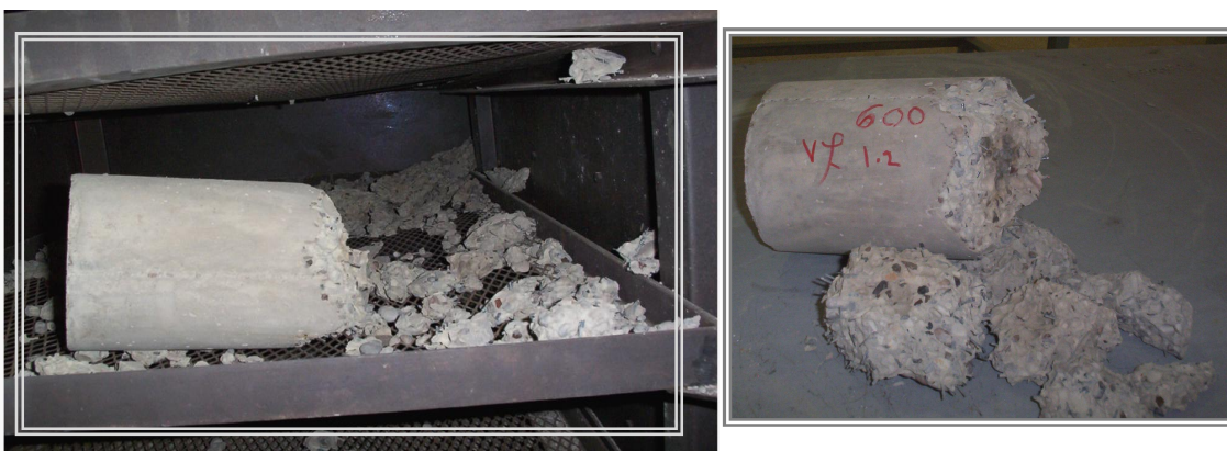
Fig. (12) Explosive spalling
